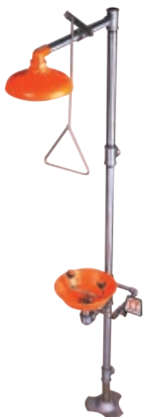
G-1902P Safety Station Consists of eye wash with ABS plastic bowl, 10" ABS shower head, stay-open push valve on eye wash and shower. Furnished with ANSI compliant identification sign.
