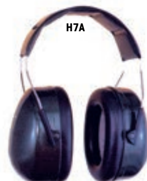
H7A Peltor Hearing Protection Padded headband, broad ear cushions, with combined liquid and foam filling to give good sealing and low surface pressure. NRR 27
